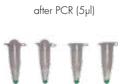
Fig. 1: Evaporation test: PCR samples were mixed with a coloured dye. Sample volume: 5 µl · Initial denaturation: 95°C; 10 minutes. Cycles: 30 · Denaturation: 94°C; 30 seconds · Annealing: 55°C; 30 seconds · Extension: 72°C; 60 seconds · Final extension: 72°C; 5 minutes. Total volume was determined before and after PCR.
