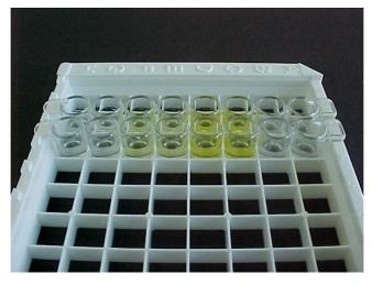
The method of Acetylcholinesterase – *Microplate Acetylcholinesterase Inhibition Assay* (**MAIA**) – for the detection of organophosphate, organochloride and carbamate pesticides residues in hydro-acetonitrilic extracts of solid/liquid food matrices is based on testing in microtitre plates of Acetylcholinesterase (AChE) activity inhibition by pesticide molecules, that belong to three important families.
