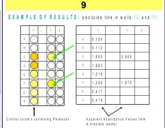
**Quantitative pesticide titers calculation** by an easy elaboration of microplate reader absorbance results.
