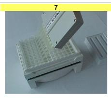
At 8' from the addition of STARTER solution to column 1, dispense 100 µL of STOPPER into every well.
