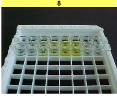
**Direct visual evaluation of pesticide titers:** Compare the colour in Sample wells with those in Control wells: a pesticide concentration estimate in the extract is obtained by the yellow colour intensity developed in the sample well, compared to the colour in control wells. The yellow colour intensity is inversely proportional to the pestice quantity.
